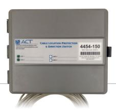
Protection System is made up of a remote switching device controlled by a Cable Location Transmitter System. In addition the ACT 445X system is built with a high-energy surge protector. The surge protector provides a low impedance path to ground for high-energy transients (Lightning, temporary over voltage TOV, etc.); and a high impedance path for low energy signals (cable locating tones).
