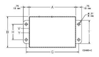
ENCLOSURE DIM L = 7.5" W= 6.28" D = 4" MOUNTING G = 6.75" H = 4.0"
